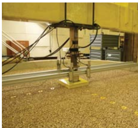
Bearing capacity tests at BRE confirm TriAx geogrids increase load distribution.
